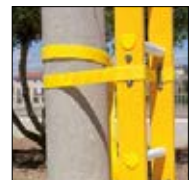
Support and anchor system
